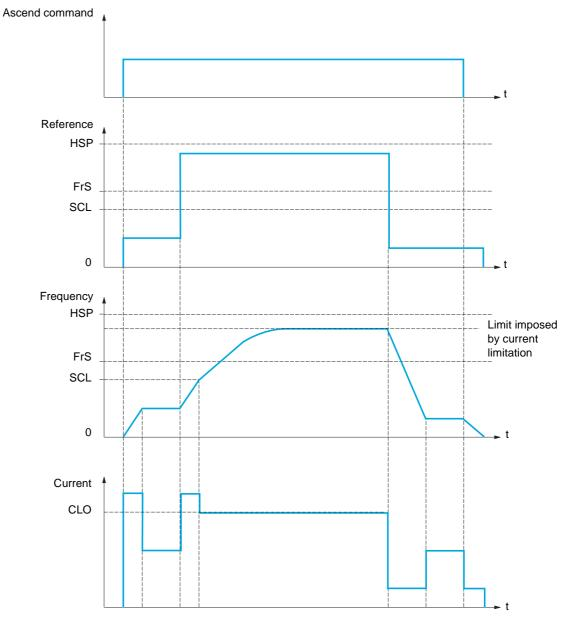
SCL: Adjustable speed threshold, above which current limitation is active CLO: Current limitation for high-speed function
