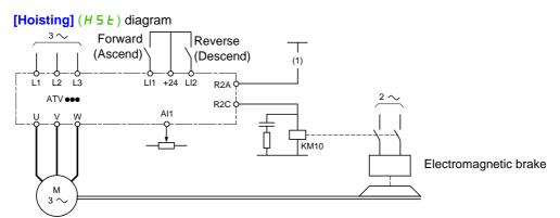
(1) Whithout integrated safety function, a contact on the Preventa module must be inserted in the brake control circuit to engage it when the "Safe Torque Off" safety function is activated (see connection diagrams in the Installation manual).
