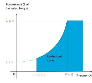
Between zero frequency and the rated frequency, the curve reflects the following equation:
