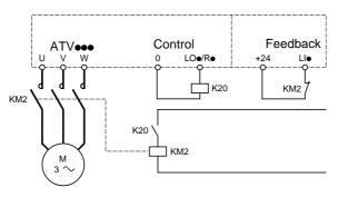
The [Out. contactor ass.] (  $\Box \ \Box \ \Box$  ) and [Output contact. fdbk] (  $\neg \ \Box \ B$ ) functions can be used individually or together.
