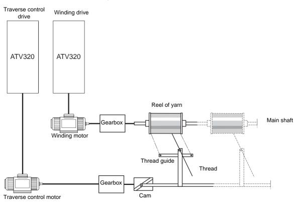
The speed of rotation of the cam must follow a precise profile to ensure that the reel is steady, compact and linear:
