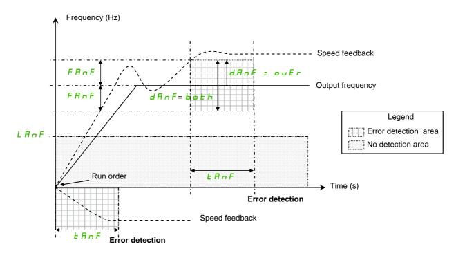
The drive will detect an error and display the error code [Load slipping] (*R*, *F*) in the following cases:
