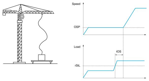
The speed step (OSP parameters) described on page 202 is used to measure the load. The effective measurement cycle will not be triggered until the load reaches the adjustable threshold [Rope slack trq level] (r 5 E L), which corresponds to the weight of the hook.
