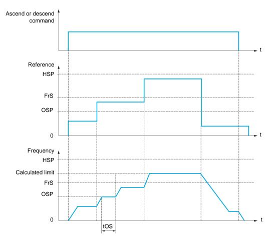
OSP: Adjustable speed step for load measurement tOS: Load measuring time
