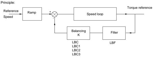
The load sharing factor K is determined by the torque and speed, with two factors K1 and K2 (K = K1 x K2).
